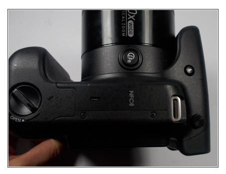
Place the camera upside down on a hard surface such as a table. Make sure that the battery compartment is visible.
