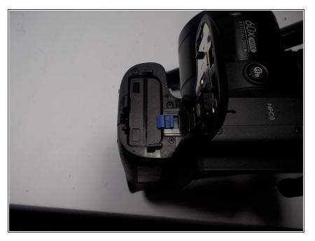
• Slide the blue tab to the right to release the battery.
