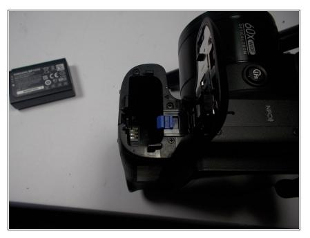
• Carefully slide the battery out of the camera. It can then be replaced with a new battery.
