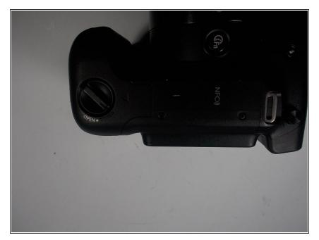
• Twist the nob counter-clockwise while pushing cover to the left. Then pull the cover up to reveal the battery.
