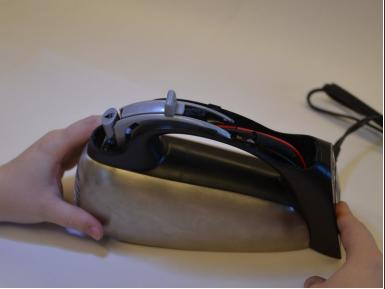
Remove the handle's cap carefully.
