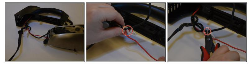
Cut zip tie holding the power cable together using handheld wire cutters.
