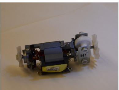
Once disconnected, the motor will slide out easily.
