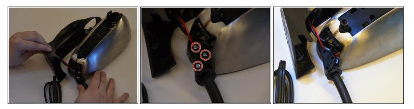
Remove the three 7.8 mm Philips #2 screws holding the power cord in place.
