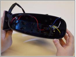
Remove the seven 5.6 mm Philips #2 screws that attach the motor casing to the mixer handle and set them aside.
