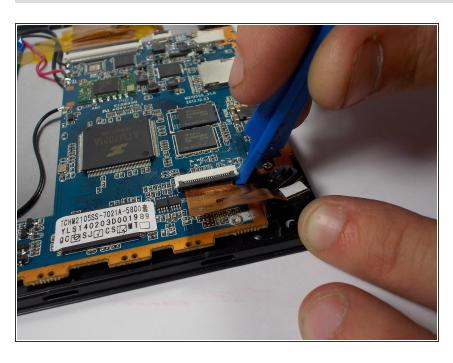
Use a smaller plastic opening tool to lift up the ZIF connector in which the cameras are plugged into.
