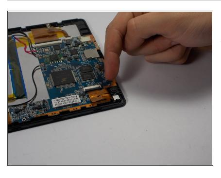
The front/rear facing cameras are located in the corner of the device one is facing toward you and is black. The other is facing away so you will see the white backing.
