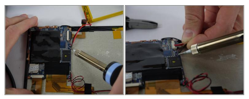
• <u>Desolder</u> the wires that connect the battery to the motherboard.
