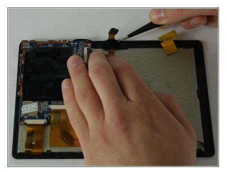
Using a pair of tweezers remove the tape securing the cameras to the back panel.
