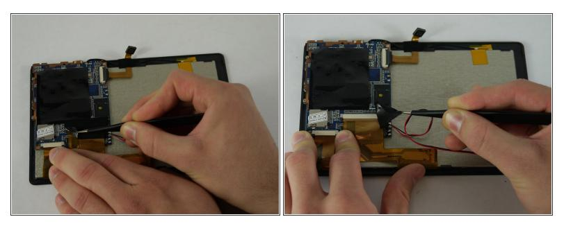
• Using a pair of tweezers begin to peel the tape covering the ribbon cable on the motherboard.
