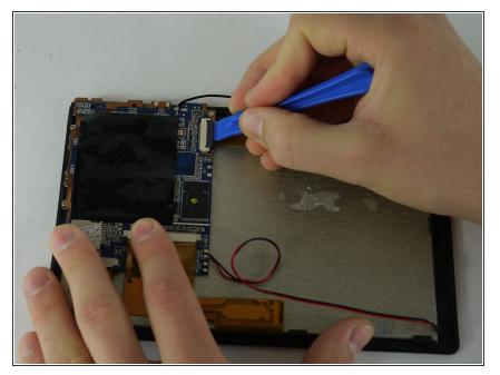
Using a plastic opening tool lift up the flap on the ribbon cable receptacle.
