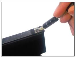
Remove the four 4.0 mm screws on both sides of the cage using a Phillips #1 screw driver.
