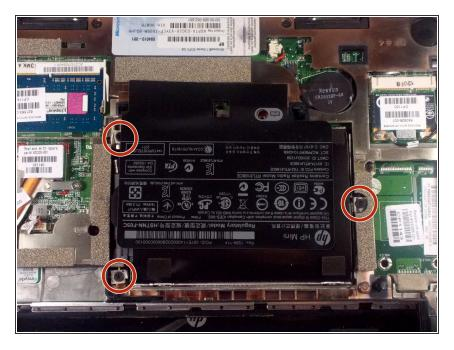
Remove the three 5.0 mm screws holding the hard drive cage in place using a Phillips #1 screw driver.
