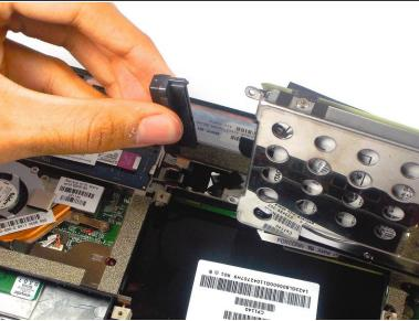
Unplug the cable connecting to the hard drive.
