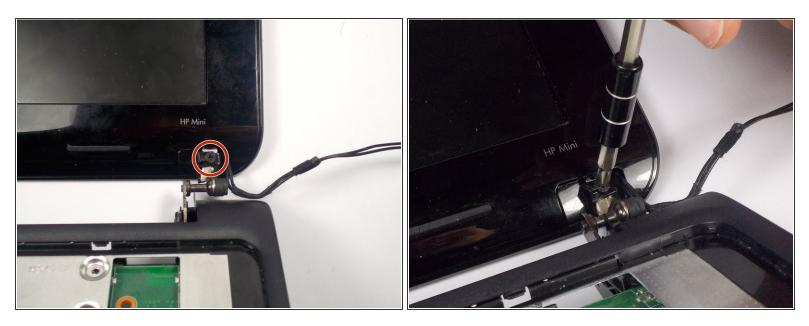
Remove the 2 3.0 mm screws on both sides of the bottom of the display using a Phillips #1 screwdriver.
