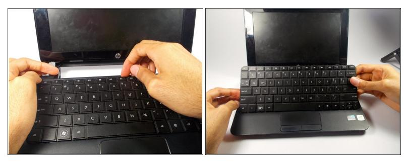
• Move and hold the bezel slightly towards the screen while lifting the keyboard from the top.
