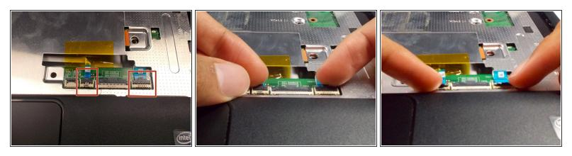
Lift the two black holders upward located next to the socket for the keyboard close to the tracked pad.
