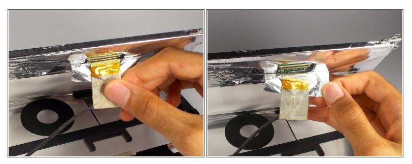
Under the screen, peel off the tape near the cable completely, so you can see the socket for the cable.
