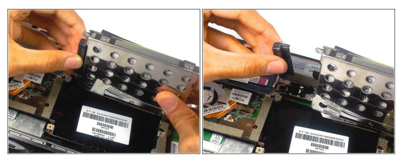
• Unplug the cable connecting to the hard drive.
