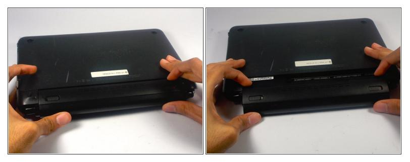
• With the left switch still pushed inward, pull the battery towards you to remove it from the computer.
