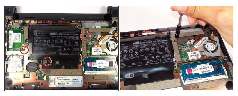
Remove the three 4.0 mm screws with the keyboard indicator next to them using a Phillips #1 screw driver.
