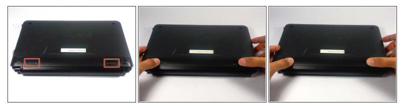
• With the bottom of the HP Mini facing up, slide both switches inward towards each other.
