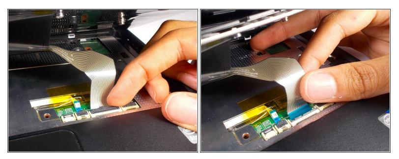
• Lift the black holder connected to the keyboard cable until it points up.
