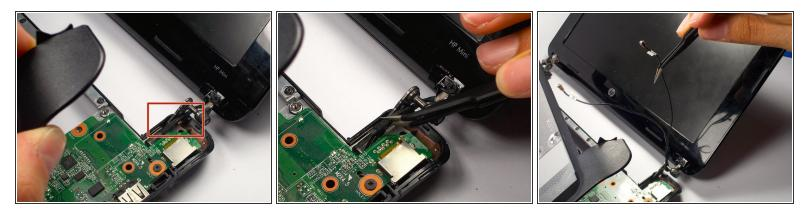
• Pull the cables for the web cam out using tweezers.
