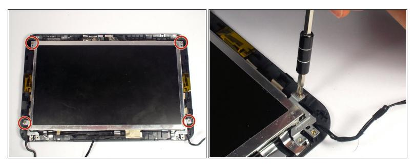
• Remove the 4 4.0 mm screws holding the screen in place using a Phillips #1 screw driver.
