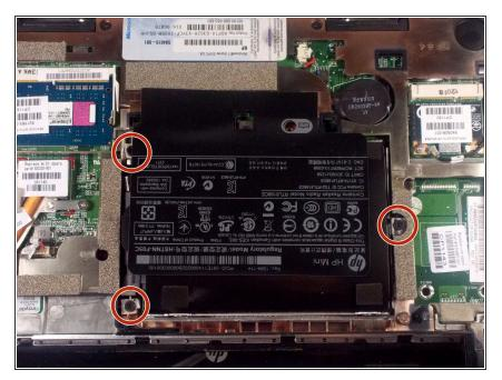
Remove the three 5.0 mm screws holding the hard drive cage in place using a Phillips #1 screw driver.
