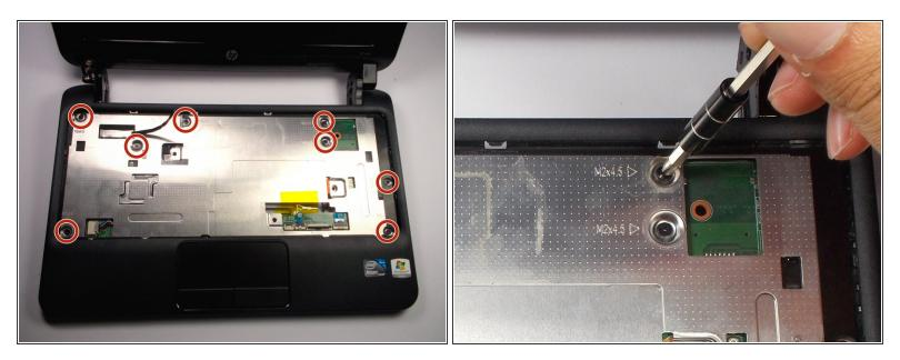
• Remove the 8 5.0 mm screws under the keyboard using a Phillips #1 screw driver.
