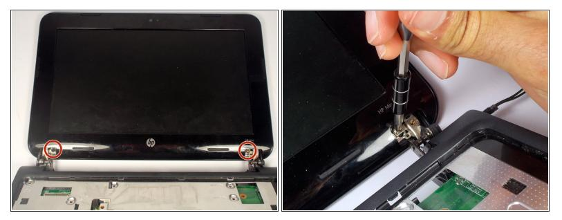
• Remove the 2 3.0 mm screws on both sides using a Phillips #1 screw driver.
