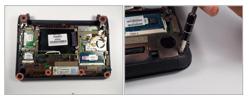
• Remove the 6 5.0 mm screws holding the back plate together using a Phillips #1 screw driver.
