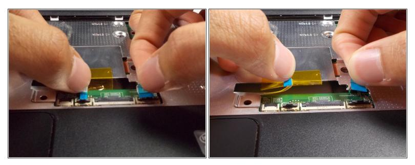
• Remove the two connectors for the motherboard from their sockets.
