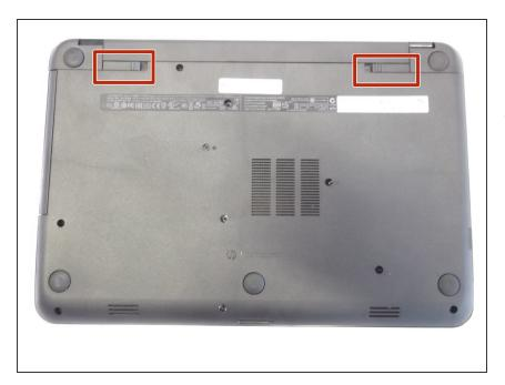
On the underside of the laptop towards the hinge for the screen there are two rectangular slide switches located inside of rectangular tracks.
