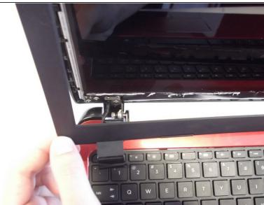
Separate the black plastic frame from the body of the computer by sliding it up and towards you while rotating the top section away from you.
