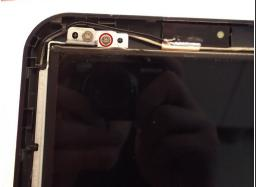
• Unscrew the 4x 4mm Phillips #1 screws from the four corners of the screen they are the ones that are attached to the metal tabs coming from the screen itself.
