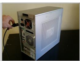
Turn off your computer and remove the power cord by pulling it straight out of its socket.
