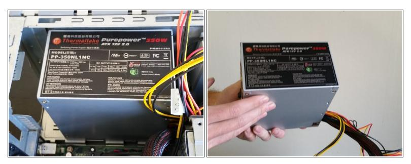
Remove the power supply by pushing it out from the back of the computer and lifting it out of the computer.
