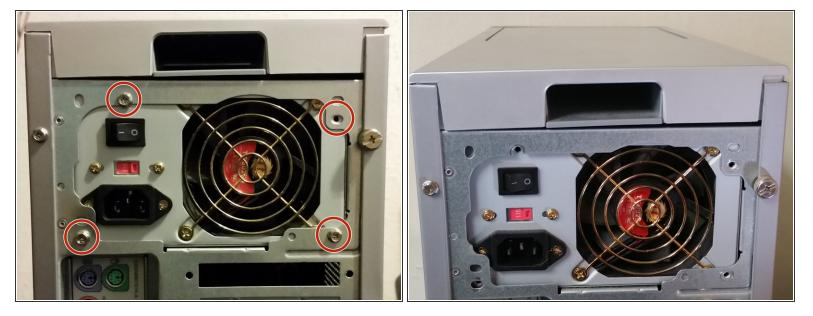
Remove the four screws holding in the power supply.
