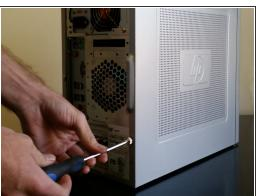
Remove the two screws holding the right (from the back) case door to the computer.
