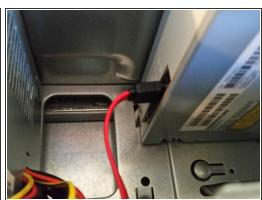
Remove the power cord from the optical disc drive by pulling it straight out.
