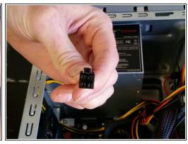
Remove the computer processor's power cord by pinching the clip on the connector and pulling it straight out.
