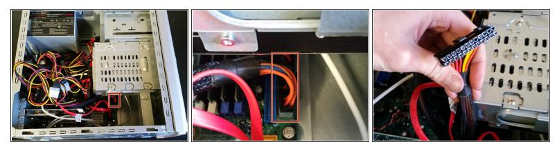
• Remove the power to the motherboard by pinching the clip and pulling it straight out.
