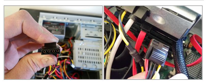
If the hard drive has a 4-pin Molex connector, pinch the two clips on the connector and pull it straight out to remove it.
