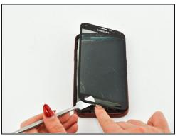
Using a plastic opening tool or spudger, pry up the screen after the adhesive has melted.
