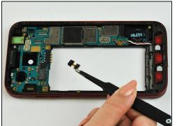
Remove the camera from the plug at the top of the phone with <u>tweezers</u>. It should pop out fairly easily.
