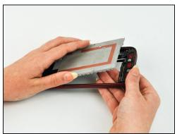
Push the plate out by applying pressure to the battery cavity.
