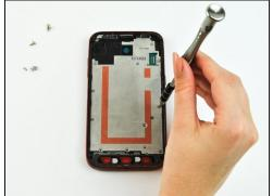
Remove the seventeen screws around the plate.
