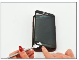
Using a plastic opening tool or spudger, pry up the screen after the adhesive has melted.
