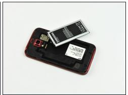
Lift up the battery using a plastic spudger or fingernail.
