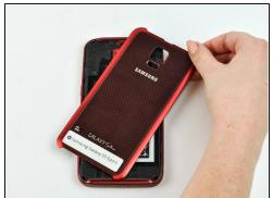
Remove the back casing of the phone using the notch located at the top.
