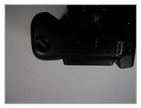
Twist the nob counter-clockwise while pushing cover to the left. Then pull the cover up to reveal the battery.
