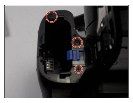
Remove the two 6mm screws located underneath the battery cover using the same screw driver with the JIS size 000 head.
