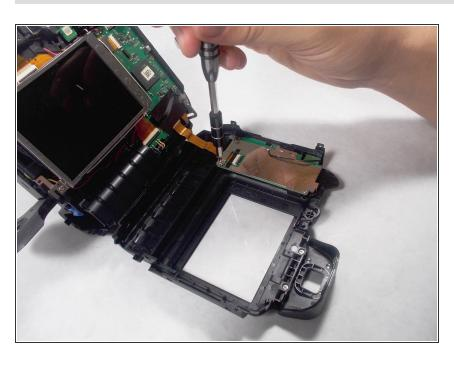
Looking at the back of the exposed face plate, remove the four 5mm screws, that hold down the metal
