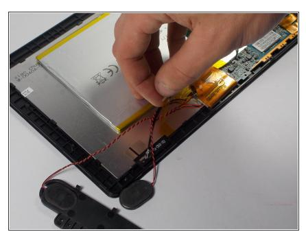
• Remove the tape holding the wires down.
