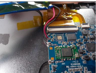
Lift up the battery it will be glued to the device.
