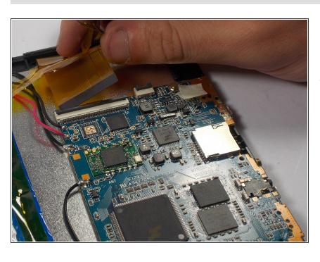
Remove the ribbon cable from the ZIF connector, it is next to the volume buttons.
