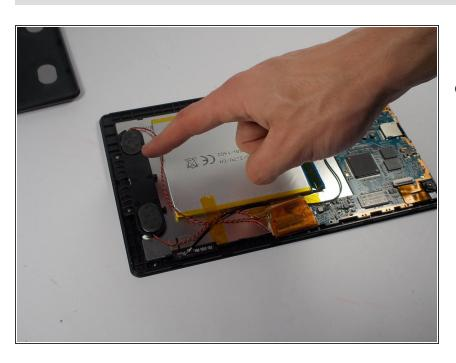
The external speakers are located in the black plastic fixture near the battery as pointed to in the image.
