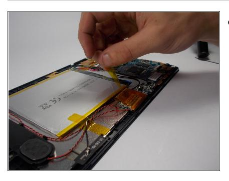
Carefully remove the tape that is holding down the battery.
