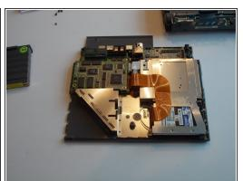
On the left side of the sisterboard, gently pull up to separate the sisterboard from the motherboard.
