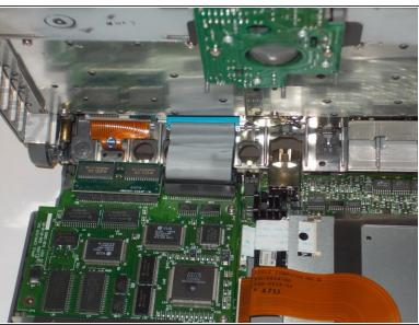
CAREFULLY lift the back of the screen and keyboard unit(the top of the computer) and GENTLY push the front left and right corners away from the bottom unit until a click is heard. Then, SLOWLY lift the top unit and remove the interconnect cable (the large somewhat brittle cable connecting the two halves) from its socket in the sisterboard.
