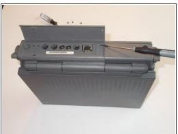
Being careful to hold the top and bottom halves of the computer together, turn to the back side of the computer and remove the final screw with a T17 Star-headed screwdriver.
