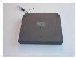
Turn the 140 upside down and remove the 4 screws in the bottom with a T10 star-headed screwdriver
