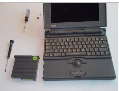
Slide the battery panel or switch(depending on your battery) toward the front of the computer, then pull the battery straight out.
