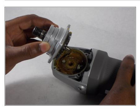
Carefully pull the head gear away from the device, and set aside.
