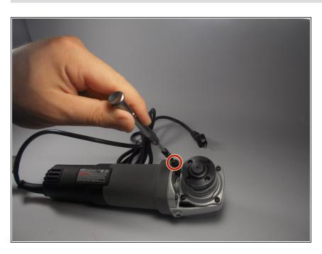
Using the Phillips #2 screwdriver, remove the 1 inch black retainer screw.
