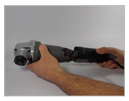
Holding the front of the device, carefully slide the back cover over the cord.
