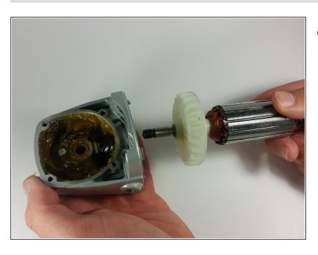
Pull the motor assembly away from the head, and set aside
