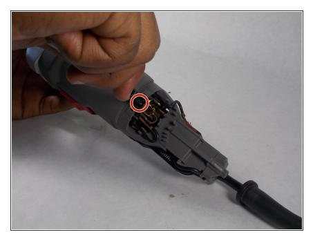
Using the Phillips #2 screwdriver, remove the 1/2" screw holding on the motor brush arm. Repeat on the other side.
