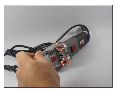
Using the Phillips #2 screwdriver, remove the other two 1/2" Phillips screws holding the head to the body on the top side of the grinder.
