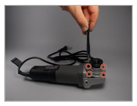
Using the Phillips #2 screwdriver, remove the four, 1/2" Phillips screws around the head gear.
