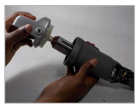
Holding the head of the device, carefully pull the motor assembly out of the body of the device.
