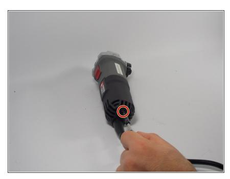
Using the Phillips #2 screwdriver, remove the 3/4" screw on the back cover.
