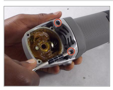
Using the Phillips #2 screwdriver, remove the two 1/2" Phillips screws holding the head to the body on the bottom side of the grinder.
