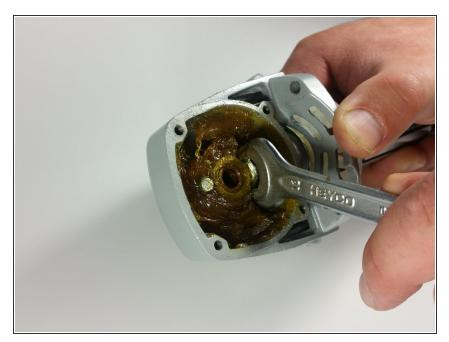
Using a 9/16" wrench, loosen the spindle nut inside the head, from the motor assembly.
