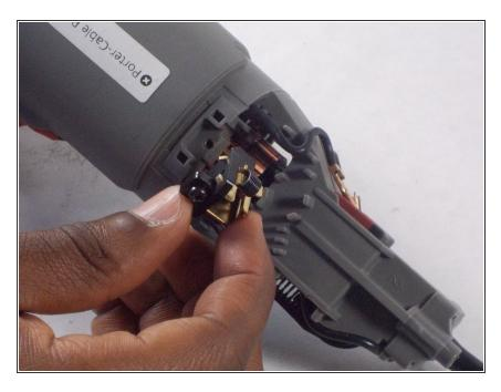
Carefully pull the motor brush arm away from the other device, you can leave the wire connected to device.
