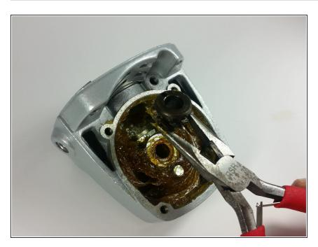
Using a pair of needle nose pliers, remove the pinion gear from the head.
