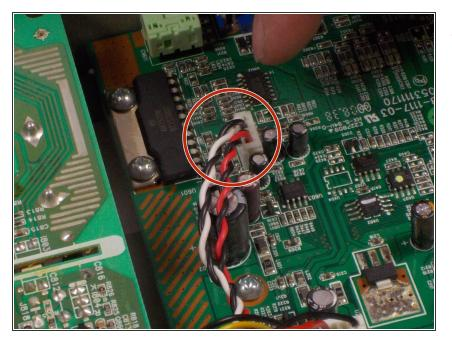
Remove the cables that connects the speakers to the signal output board.
