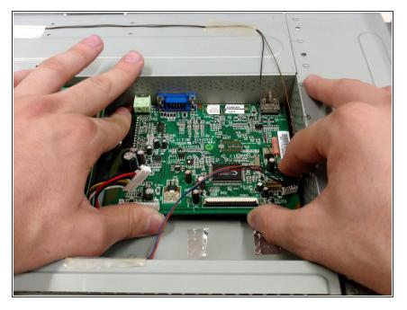
Lift the board out of the screen assembly by first pulling the board away from the wall where the ports mount, then upward.
