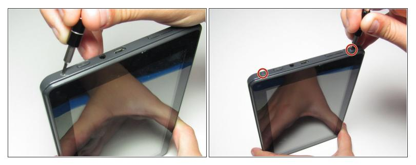
• Remove the two 5mm screws from the bottom of the device using a Phillips #000 screwdriver.
