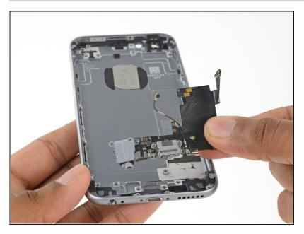
Remove the Lightning connector and headphone jack assembly.
