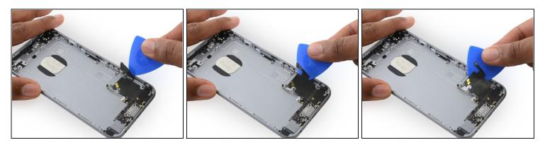
• Insert an opening pick between the Lightning connector assembly and the rear case to begin breaking up the adhesive holding the flex cable in place.
