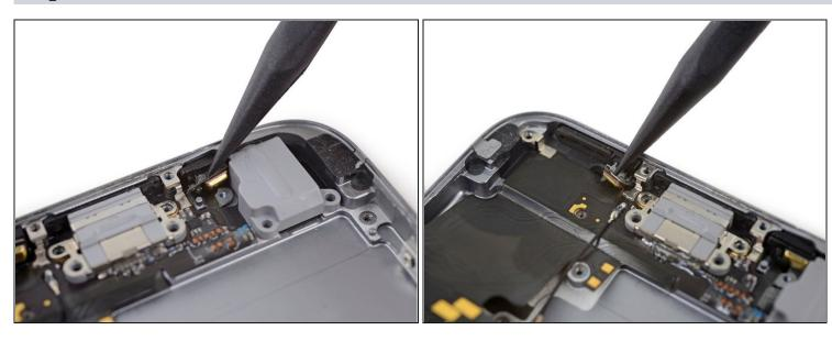
• Use the tip of a spudger to separate the two microphones from the lower edge of the rear case.
