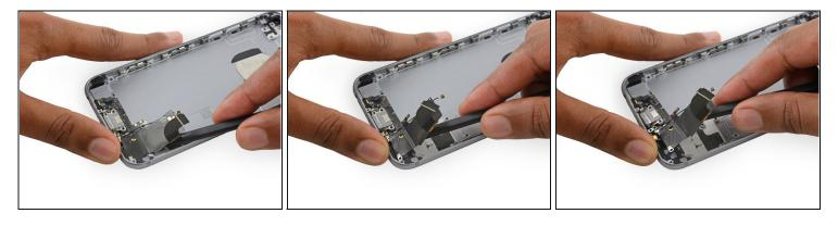
• Use the flat end of a spudger to continue separating the Lightning connector assembly from the rear case.
