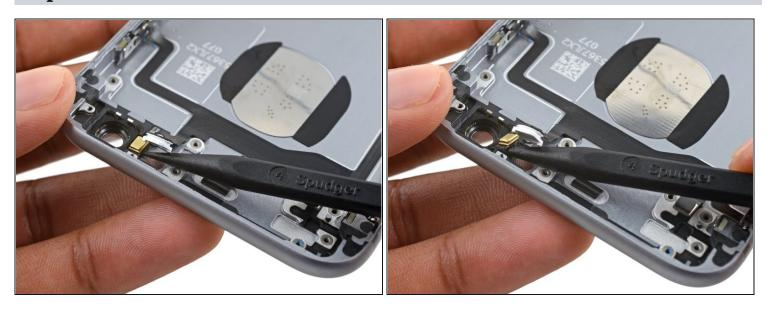
• Use the pointed tip of a spudger to gently separate the microphone from the rear case.
