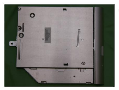
Remove the optical drive, if all the screws have been removed is should slide out easily.
