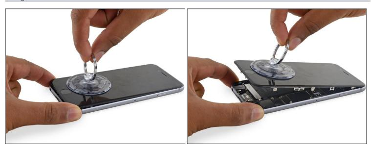
• Use the suction cup to open the display, breaking the last of the adhesive.
