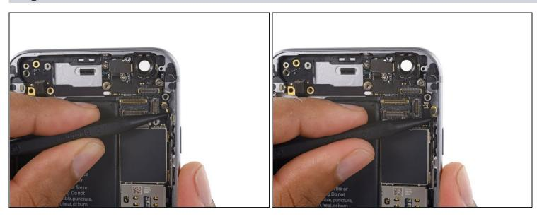
• Use the pointed tip of a spudger to disconnect the antenna cable from its socket on the upper right corner of the logic board.
