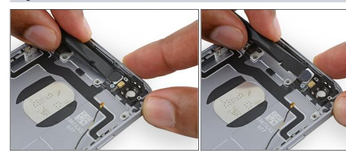
• Use the flat end of a spudger to lift the flash out of its housing in the rear case.
