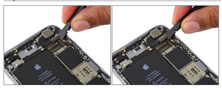
• Use the flat end of a spudger to disconnect the rear camera from its socket on the logic board.
