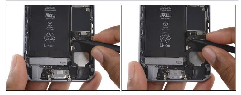
• Use the pointed tip of a spudger to disconnect the antenna cable from its socket on the lower left corner of the logic board.
