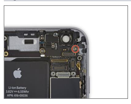
Remove the 1.3 mm Phillips screw securing the NFC bracket to the logic board.
