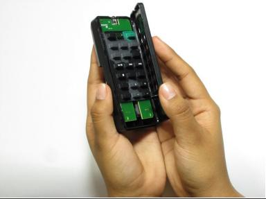
Carefully remove the top to reveal the button covers and the remote control board.
