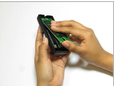
Lift the chip out of the plastic casing to replace it.
