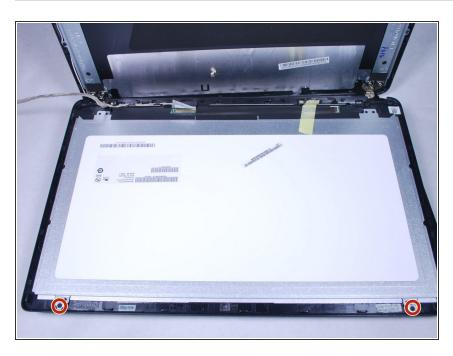
Remove the two brackets holding the displays by unscrewing both M1 .6x3 screws with a PH0 Phillips screwdriver.
