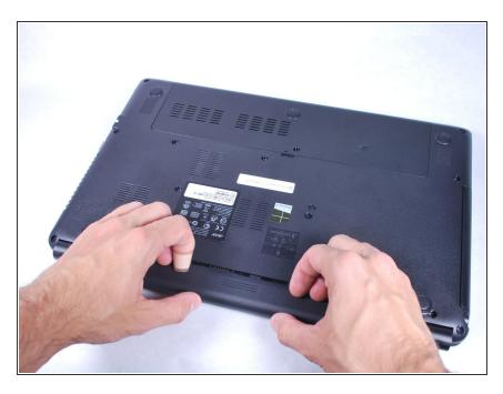
Firmly grab hold of the battery and slide it out of the laptop.
