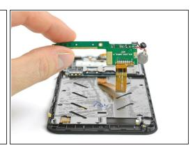
After lifting the vibrator and the microphone carefully out of their recesses we free the daughterboard by loosening two more Phillips screws.
