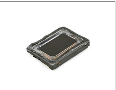
Before we take the frame aside we take a short look at the loudspeaker which is embedded with a mild double sided adhesive tape.
