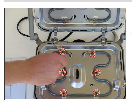
Remove the six 5.5mm Phillips #2 screws that secure the bottom heating coil to the device.
