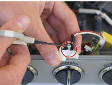
• Cut the zip ties which hold the LED lights in place with scissors/knife.
