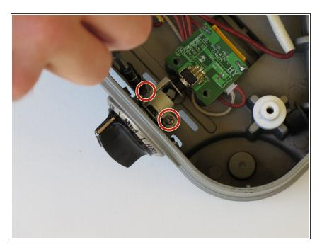
Remove the two 6 mm Phillips #2 screws that secure the white plastic LED holder.
