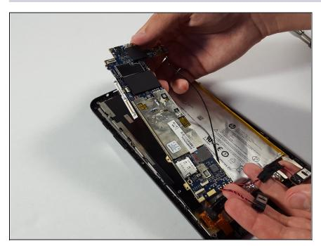
Remove the motherboard from the device.
