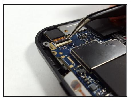
Lift up on the small black tab at the connection point to unlock the flex ribbon cable using the <u>tweezers</u>.
