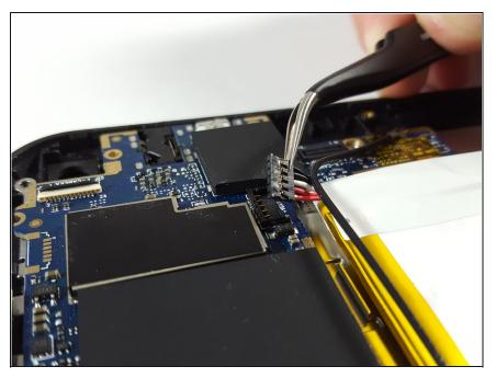
• Carefully remove the battery connector from the system board using the <u>tweezers</u>.
