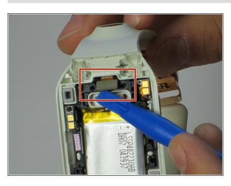
Loosen the camera ribbon so it will easily pass through the watch body.
