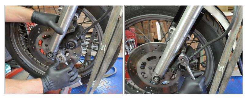
• Using a torque wrench, tighten both screws to between 25 and 30 foot-pounds.
