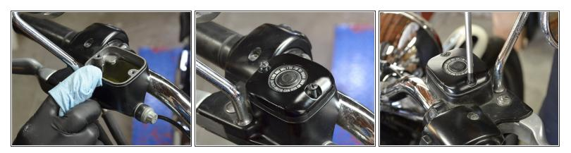
• To prevent spilling any brake fluid, first clean the area around the master cylinder with a clean rag, then replace the cover.
