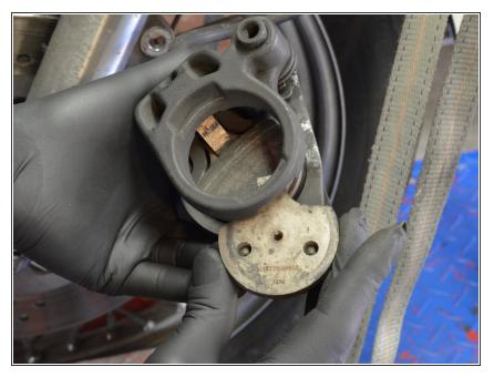
Being careful to not let any loose parts fall out of the brake assembly, remove the stationary brake pad from the front brake assembly.
