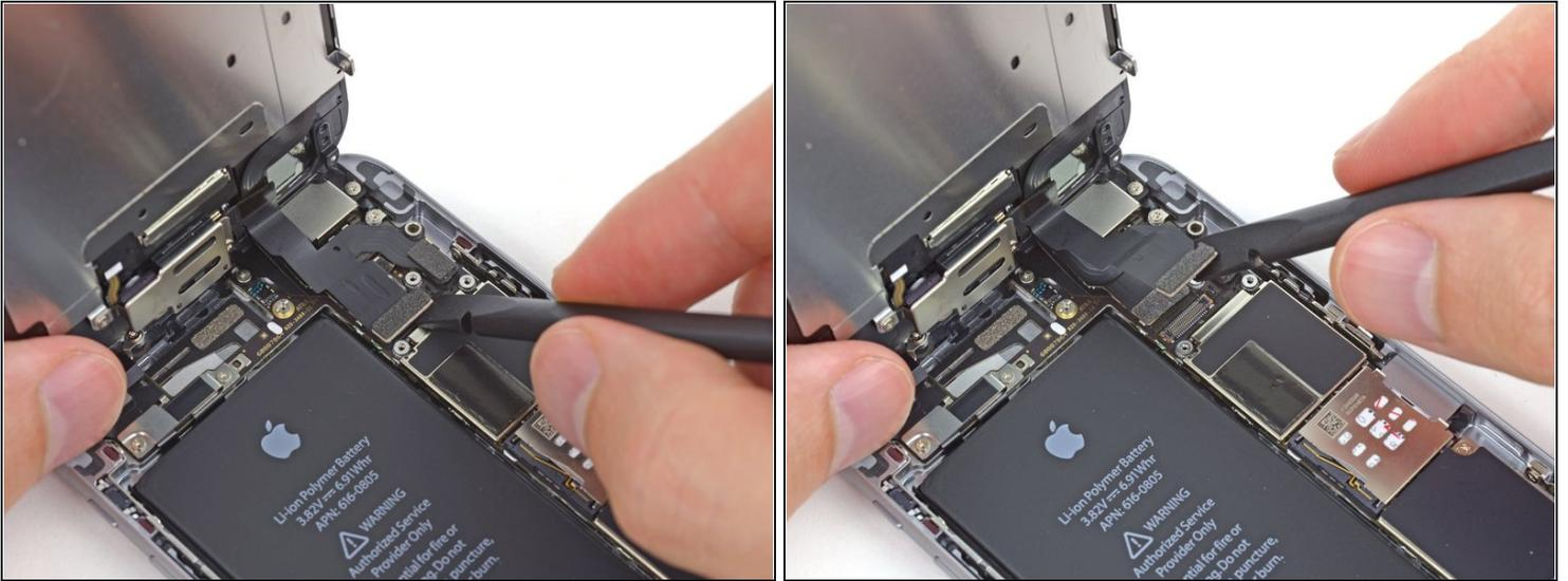
⚠ In the next four steps, take care to pry up **only** on the cable connectors, and not on their sockets on the logic board.
