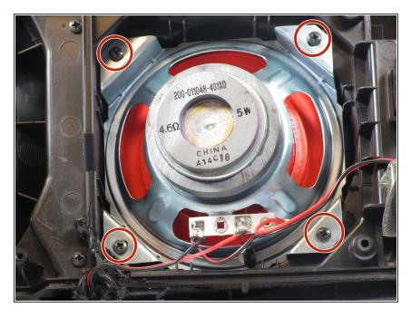
Use a Phillips #2 screwdriver to remove the 1/2 inch screws.
