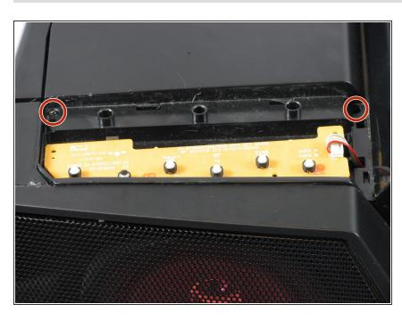
Use your Phillips #2 screwdriver to remove the two 1/2 inch screws underneath the now-removed panels.
