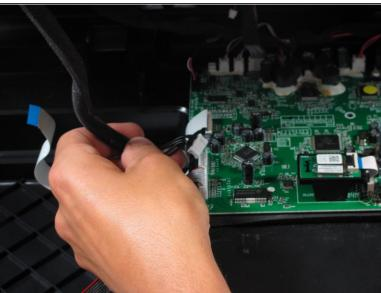
Disconnect the antenna cables.
