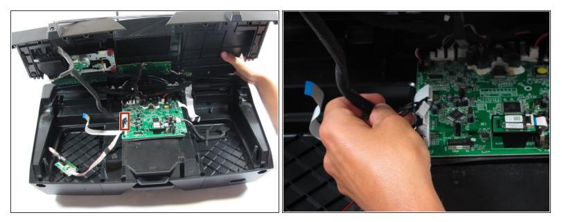
Disconnect the antenna cables.
