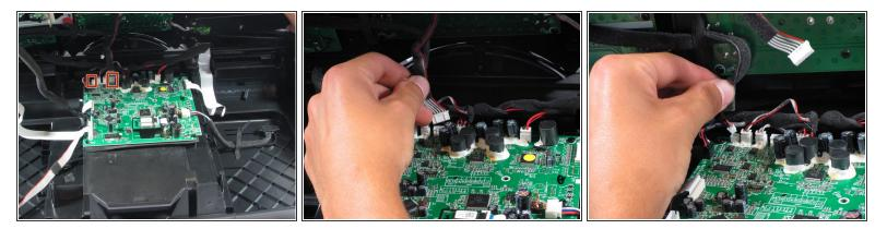
Disconnect the remaining cables from the motherboard.
