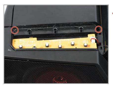
Use your Phillips #2 screwdriver to remove the two 1/2 inch screws underneath the now-removed panels.
