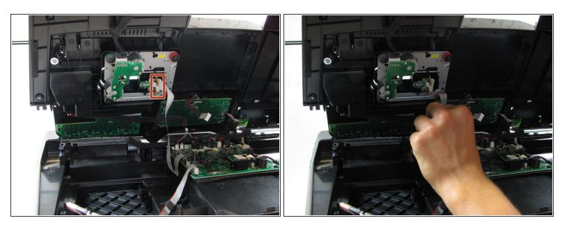
Disconnect the CD drive ribbon cable from the top of the device.
