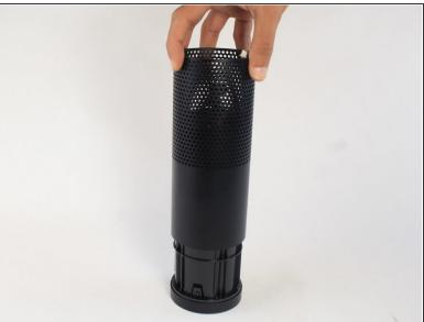
Remove the plastic plate from the bottom of the device. Then remove the plastic shrouding.
