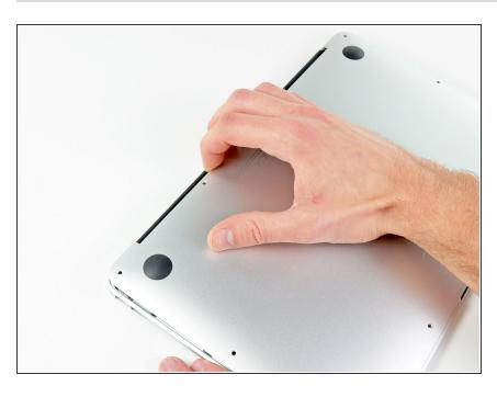
Wedge your fingers between the display and the lower case and pull upward to pop the lower case off the Air.
