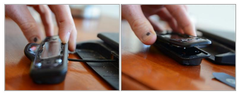
• The little plastic screen part just popped out. Just wiggle it loose with a small screwdriver. Then there are just four screws to remove (regular Phillips #2) and you're in!
