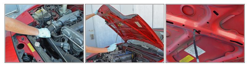
• With the hood raised, insert the hood prop into the hole marked "rod" on the inside of the hood.
