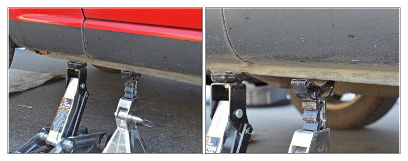
• Place your jack back in the same location on the frame you used to jack up the car. Raise the jack until it touches the jacking point on the frame.
