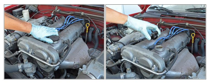
• Remove the oil filler cap at the front of the engine by twisting it counter-clockwise and then lifting it up.
