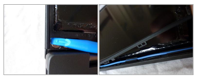
• Remove the rear bezel with the prying tool.
