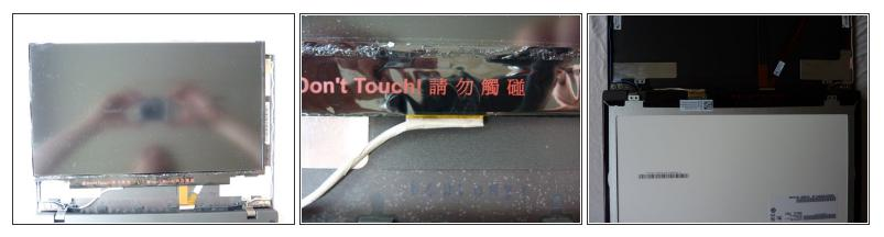
• Carefully release the display, turn it around and place it on the keyboard.
