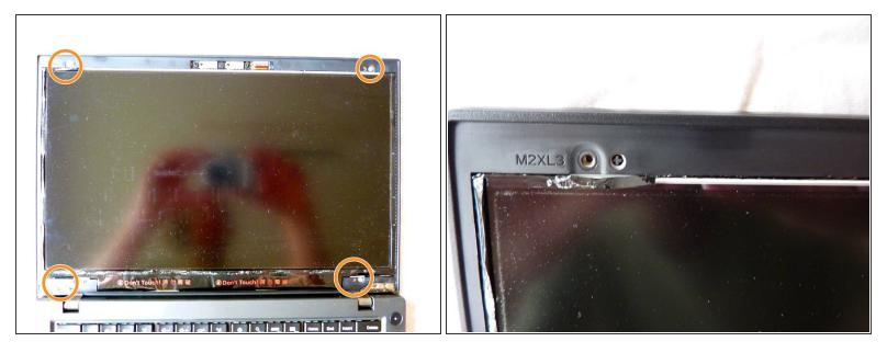
• Remove 4 screws **M2XL3** with screwdriver.
