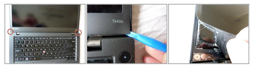
• Start removing the front bezel in the lower display corners using a prying tool.
