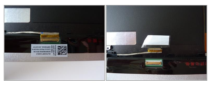
• Remove the connector together with the label.
