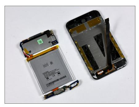
The logic board and battery can now be fully separated from the rest of the iPod.
