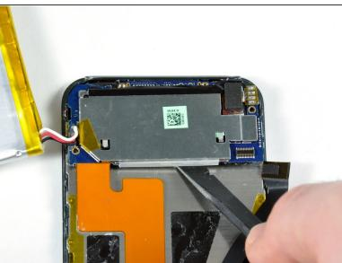
Use the spudger to loosen the logic board from multiple sides. It is held in place by glue and the four screws that were removed in the previous step.
