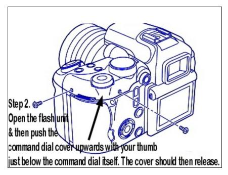
Remove the command dial cover by pushing the cover upwards with your thumb just below the command dial.
