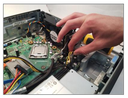
Pull out the yellow and black connector that is connected to the Motherboard.
