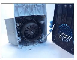
• Next you will need to tip the mixer onto its back to get a better angle. After you tip it onto its back, you will need to take a screwdriver with a 9/32 head or a 9/32 socket and unscrew the four bolts thus removing the black bottom tray.
