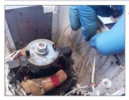
After you remove the first connection, this motor brush will begin to come out but do not remove it completely.
