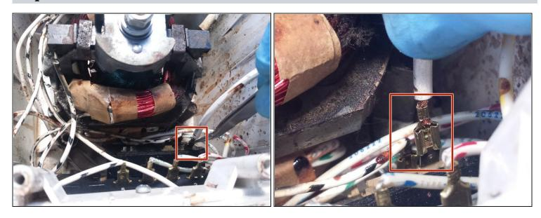
• Lastly you will need to use tweezers or needle nose pliers to remove the last electrical connection. With this connection all you need is to pull back on the metal part or the connection with your tweezers or needle nose pliers.
