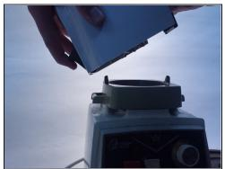
• To begin you need to remove the top of the blender. To do this you must push inward on the tab located on the bottom of the top half of the machine. After pushing the tab you can then lift up using the handle to remove the top.
