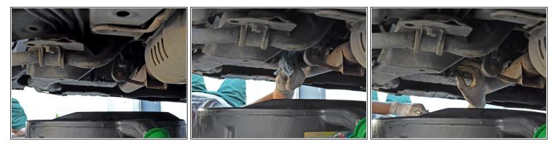
• When the oil drain has halted, or slowed significantly (drip...... drip...... drip), wipe its chin with a clean paper towel or rag.
