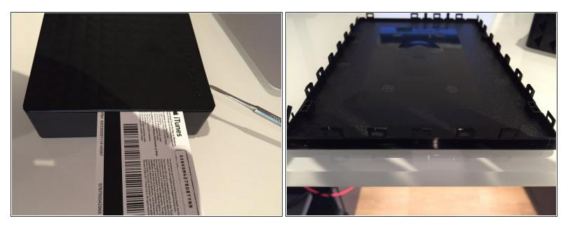
• Use the metal spudger to open up the device gently, then slide in a credit card and work around the drive gently prying (push the card in to push the clips in and stop them breaking)
