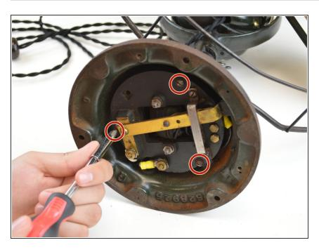
Remove the three number 8 screws that hold the switch in place.
