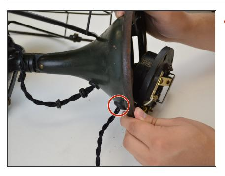
Remove the switch and set it aside, then pull the wire through the grommet.
