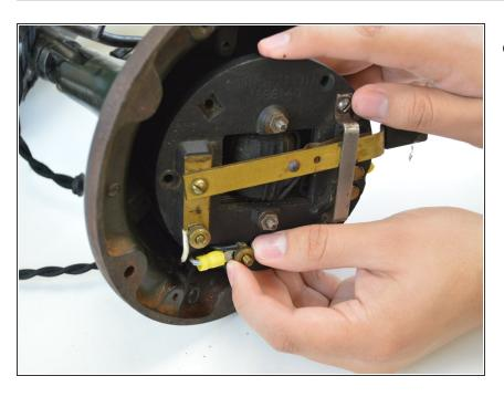
Once the switch is free, unscrew the two knurled nuts holding the wires in place.
