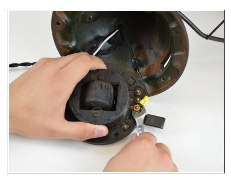
Turn the switch over and unscrew the nut securing the wire with the 5/16 crescent wrench.
