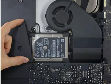
Remove the left and right hard drive brackets from the iMac.
