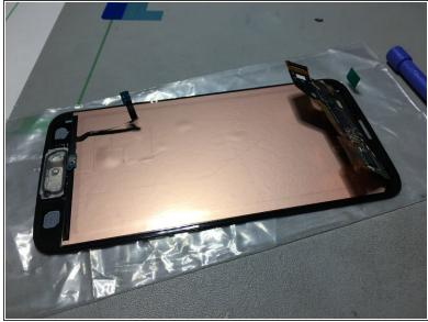
Prepare your screen assembly by removing adhesive film. If you're not replacing the screen then you can skip this step.
