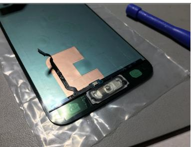
Attach the home button to the screen assembly. In this guide I am also installing a new screen assembly.
