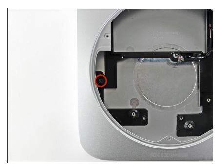
Remove the 7.9 mm T6 Torx screw securing the hard drive tray to the outer case.
