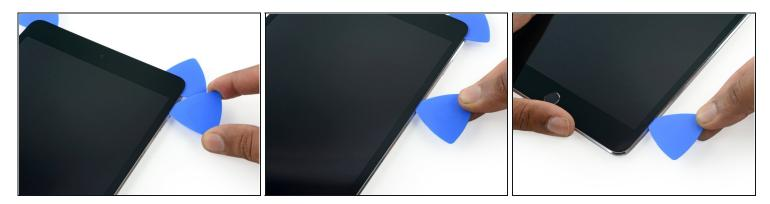
• Continue sliding the opening pick down the right edge of the iPad, reheating the edge using an iOpener if necessary.
