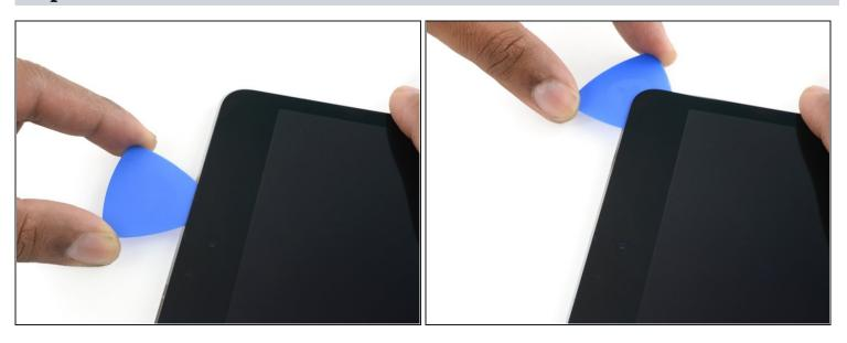
• Insert the previous pick deeper into the iPad and slide it away from the camera toward the corner.
