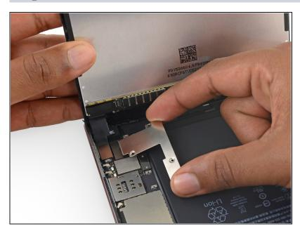
• Remove the battery/display cable bracket.
