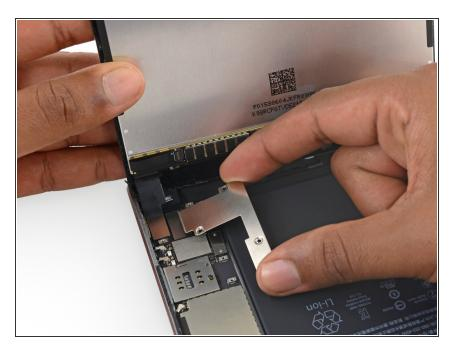
Remove the battery/display cable bracket.
