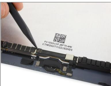
Use the pointed tip of a spudger to flip up the retaining flap on the home button ZIF socket.
