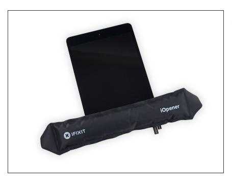
Heat an iOpener and lay it over the lower edge of the front panel to soften the adhesive holding the home button in place.
