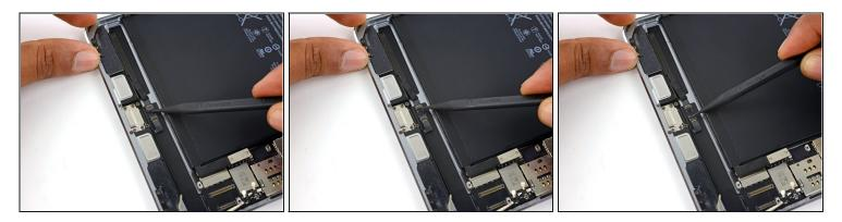
• Use the tip of a spudger to lift each of the two ZIF connector retaining flaps.
