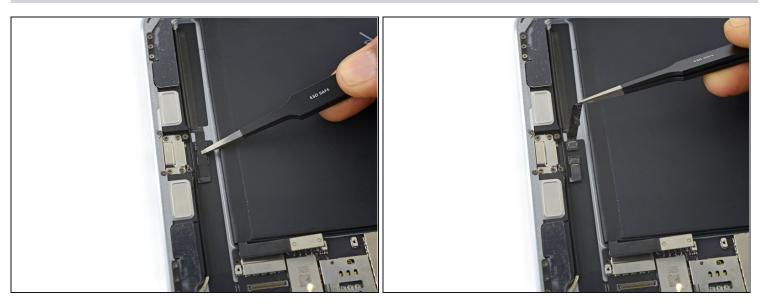
• Remove any tape covering the ZIF connectors near the Lightning connector port.
