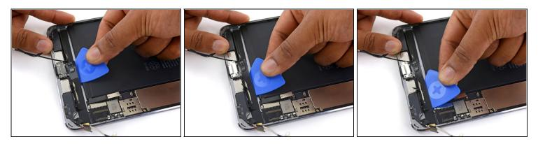
• Use an opening pick to separate the adhesive connecting the lightning connector cable to the iPad case.
