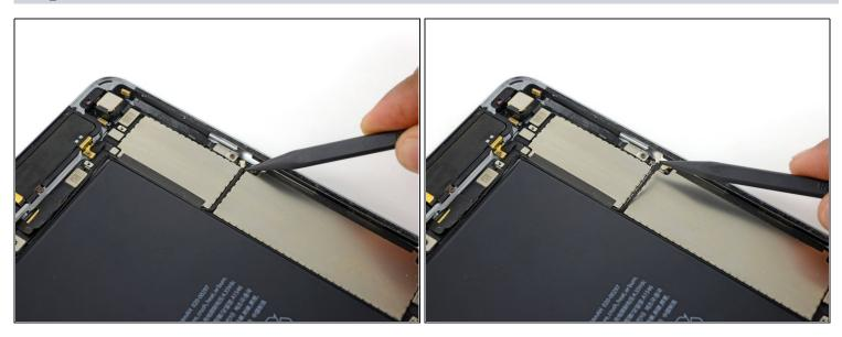
• Use a spudger to disconnect the upper antenna interconnect cable from its socket on the logic board.
