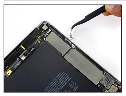
• Remove the volume control cable bracket.
