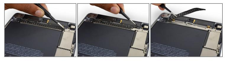
• Use tweezers to peel up the looped tape adhered over the upper component cable bracket.
