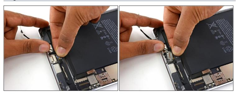
• Begin to gently lift the Lightning connector cable up.
