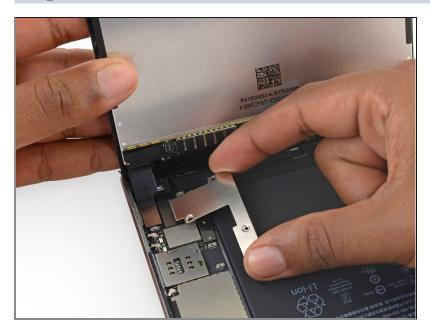
• Remove the battery/display cable bracket.
