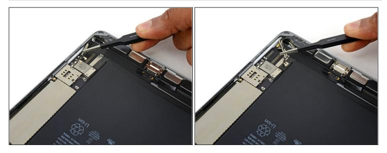
• Peel the lower antenna interconnect cables away from the corner of the rear case.
