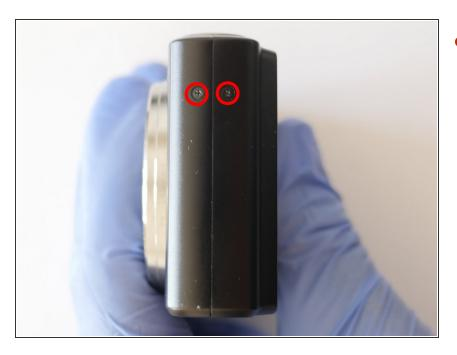
Remove 2 (0.3mm) screws from the left side of the camera.
