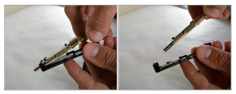
• Lift the back of the motherboard and slide it out of the case.
