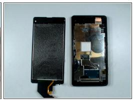
Disconnect the display assemble flex cable.
